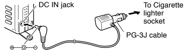
**CAUTION:** TO CONNECT AN EXTERNAL 24 V POWER SOURCE VIA A DC-DC CONVERTER, ONLY USE THE PG-3J CIGARETTE LIGHTER CABLE. USING THE PG-2W DC CABLE IN THIS SITUATION MAY CAUSE A FIRE.
